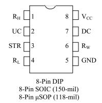
The DS1809 is available in standard 10 k $\Omega$ , 50 k $\Omega$ , and 100 k $\Omega$  resistor versions. The DS1809 is provided as an industrial temperature grade part only. Available packaging for the DS1809 include an 8-lead (300-mil) DIP an 8-lead (150-mil) SOIC, and an 8-lead (118-mil)  $\mu$ SOP.
